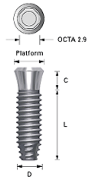
Fig. 2. The schematic of domestic Osstem implant. with 4.1mm in diameter, 13mm in length of SSII(internal hexagon connection) implant fixture.
