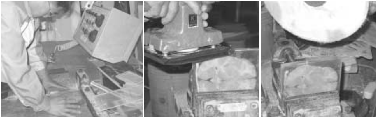
Fig. 12. Trimming of margins of the permanent specimen using electric acrylic cutter (left); grinding of surfaces of the permanent specimen using electric sandpaper machine (center) and subsequently using electric polishing machine (right).
