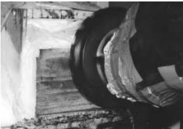
Fig. 3. Cryomacrotome on which embedding box is serially sectioned by rotating cutting blade to make a sectioned surface.
